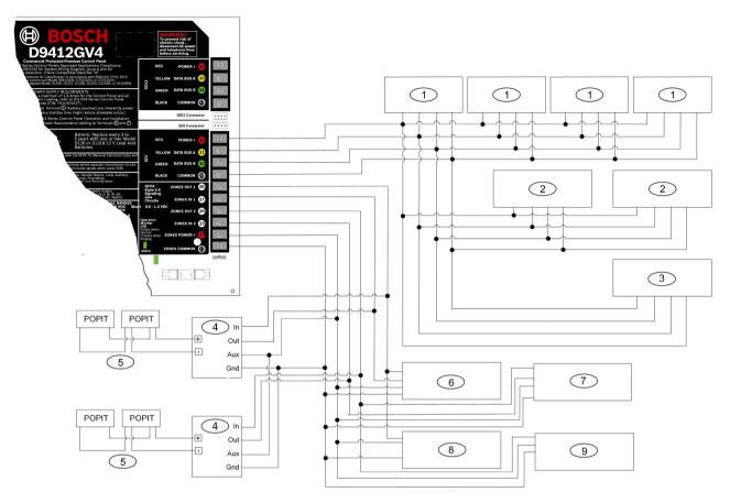
Figure 3.4: D9412GV4 System Wiring Diagram, SDI and Zonex Devices
